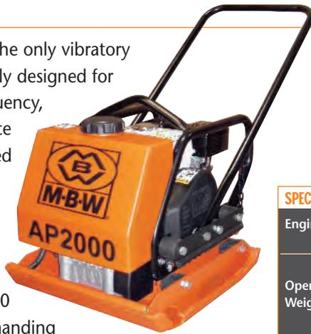
Further, the mechanical construction of the AP2000 is specific to this very demanding application. Stress relieved steel plate housings are crack resistant and provide long wear. Aluminum exciter housing dissipates heat rapidly and custom lubricants preserve bearing and seal integrity. The self cleaning plate prevents dirt build-up.
