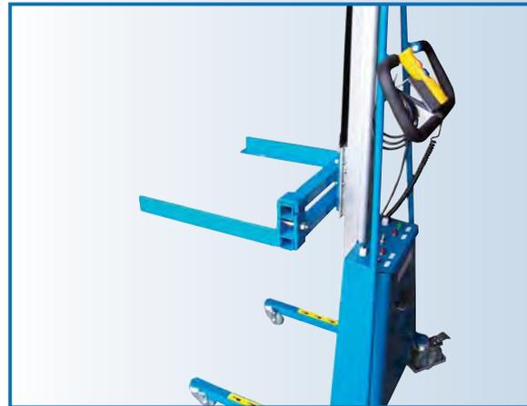
Attachment A-5 is the *Tote Lifter*. Ideal for order picking, placing totes on or off conveyors or packing stations. It can handle a tote with a maximum bottom size of 18" W x 24" L. The maximum top width is 21". The capacity with this attachment is 125lbs. Note the tote must have a lip strong enough to support the load. Contact our factory for more information.
