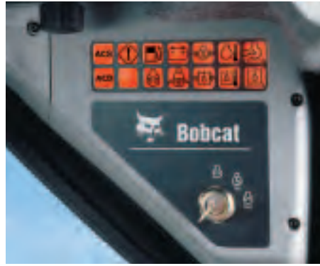
Right Side Standard Instrument Panel
